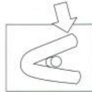
5. Tying the cap over the fence panel is done using the original 3 wire ties cut in half and tied to the outside structural wires in 4 places. Once these 4 wires are attached to the outside on one side of the cap, position the rounded cap over the fence panel. Push the ends of the 4 loose tie wire through the fence panel, then pull the wires tight and twist each of the 4 tie wires to the outside structural wire on the other side of the cap.
